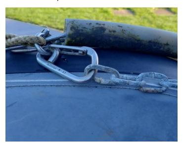
To moor the boat, release the carbine hook from its storage place on the eye in the floor of the boat. The chain is encased in a clear plastic pipe and is permanently attached to the Dring on the outside of the boat under the bow. Then lift the mooring buoy onto the side of the boat and attach the carbine hook to the chain below the buoy. Lower the mooring buoy back into the water.
